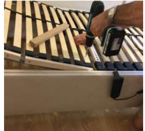
The first step is to screw the two battens supplied, to the underside of each of the two slats.
