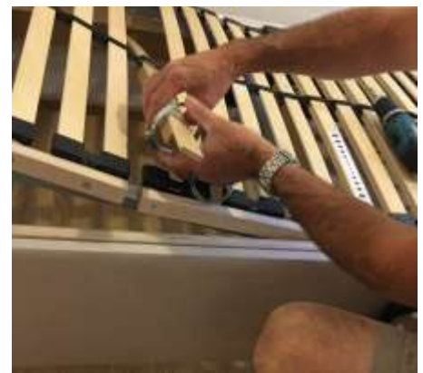
Slip a jubilee clip over each end of the two slats.
