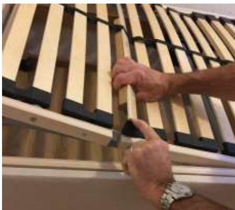
At the same time, twist the slat and it will come out.
