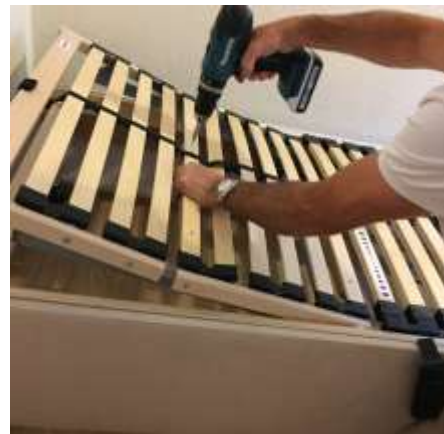
Screw through the slat into the batten approximately 5cm from each end of the batten.
