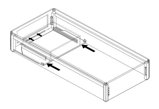
ENSURE THE BASE PANEL SITS ABOVE THE FOOT END SUPORT BATTEN AND HARD UP AGAINST THE FOOT END PANEL.IF THERE IS A GAP ON EITHER SIDE, CHECK THE BASE CORNERS ARE SQUARE (SEE PAGE 12)
