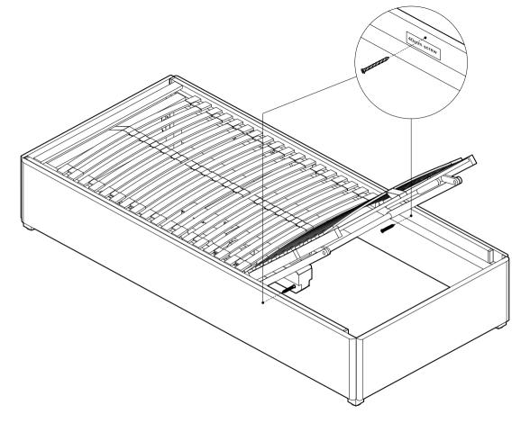
SECURE THE MECHANISM TO THE BASE USING THE 2 X 40MM SCREWS SUPPLIED. IF THERE ARE NO LABELS OR PRE-DRILLED HOLES FOR THESE SCREWS, SIMPLY SCREW THROUGH THE PLYWOOD INTO THE BASE APROXIMATELY WHERE SHOWN IN THE DIAGRAM
