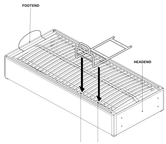
$5^{\text{TH}}$  -  $10^{\text{TH}}$  SLAT FROM HEADEND CAN BE PLACED ON EITHER SIDE OF THE BED
