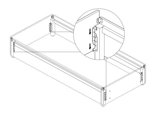
IF THE TONGUE OF ANY OF THE INTERLOCKING BRACKETS HAVE BECOME BENT, IT MAY BE NECESSARY TO USE A FLAT SCREWDRIVER TO LEVER IT OPEN TO ALLOW A GOOD FIT
