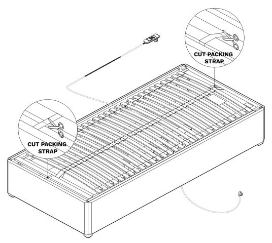
IMPORTANT: CUT THE PACKING STRAPS AT EACH END BEFORE ATTEMPTING TO RAISE THE HEAD OR FOOT SECTIONS.
