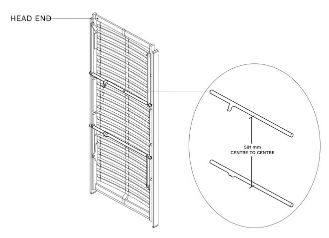
IT IS EASIER TO FIT THE MOTORS WITH THE MECHANISM STOOD VERTICALLY.
