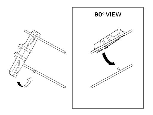
PUSH THE FOOT END ONTO THE FOOT END DRIVE BAR. THIS SHOULD CLICK WHEN LOCATED.
