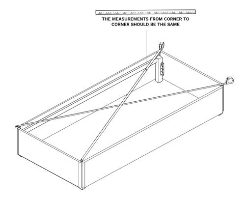
TO ENSURE THE CORNER ANGLES ARE EQUAL, THE DIMENSIONS FROM CORNER TO CORNER SHOULD BE THE SAME. IF THEY ARE NOT, DRAWERS AND MECHANISMS WILL NOT FIT CORRECTLY.
