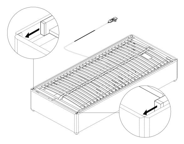
PULL THE MECHANISM DOWN TO THE FOOT END. IF THERE IS A GAP BETWEEN THE MECHANISM AND THE FOOT END OF THE BASE ON EITHER SIDE, CHECK THE BASE CORNERS ARE SQUARE (SEE PAGE 12)
