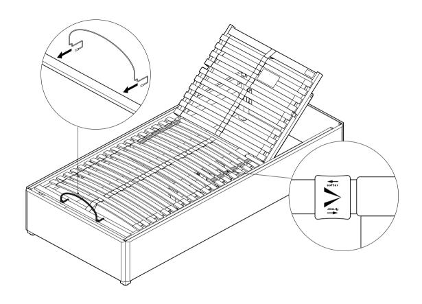
MORE FORCE IS EXCERTED IN THIS SECTION WHEN THE HEAD END IS RAISED. SLIDE THE TENSIONERS TO THE OUTSIDE TO MAKE THE SEATING SECTION FIRMER. THIS CAN BE SOFTENED IF REQUIRED BY SLIDING THE TENSIONERS TOWARDS THE MIDDLE
