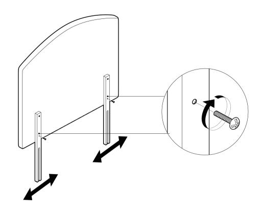
LOOSELY FIT THESE TWO BOLTS TO ALLOW THE STRUTS SOME MOVEMENT MAKING IT EASIER TO POSITION.
