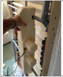
Position the twin motor over the hooks of the drive bars.
