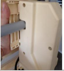
Slide the motor covers back on. They will not fit if the motors are not pushed back on hard enough.
